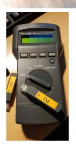
Another pair was slightly high on impedance. The fault was also showing as being only 3m from the test meter. Cable map testing confirmed the distance to fault, and also the total length of the cable run (29m).
